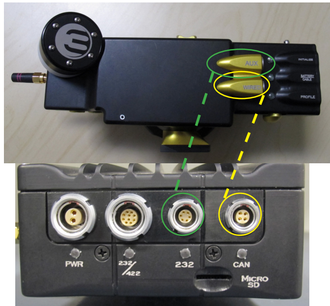
Figure 6.1a Connect from Wired port on THC to RS232 on 6-axis box.
