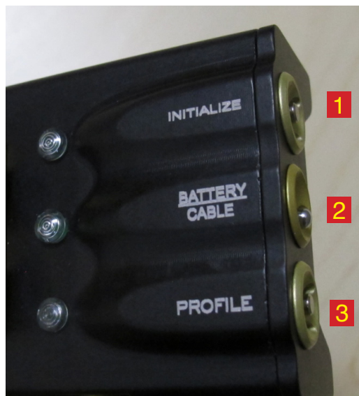
Figure 10.2a 1) Initialize button, 2) Battery/Cable switch, 3) Profile button
